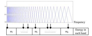
Fig. 3. Frequency response of a typical Mel-scaled triangular filter bank.
