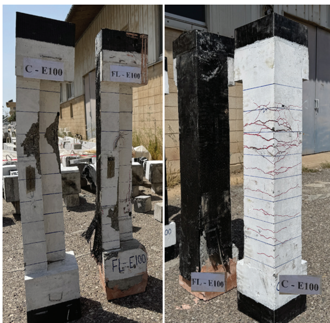
Fig. 8. Mode of failure and crack pattern of column specimens ( e_x = e_y = 100 mm).
