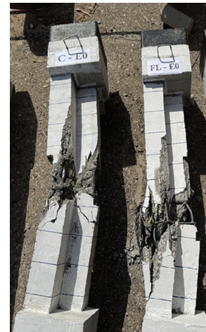
Fig. 6. Mode of failure of column specimens ( e_x = e_y = 0 ).
