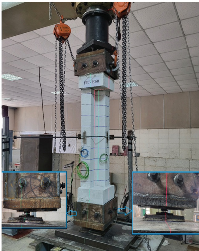
Fig. 5. Set up of the column specimen, the loading plates and steel balls that can be set in x and y directions using a self-leveling digital laser to provide a certain eccentricity with respect to the longitudinal axis of the column are indicated by the blue frames.
